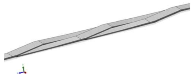
Fig. 5 3D representation of the transposition section of three Roebel strands
